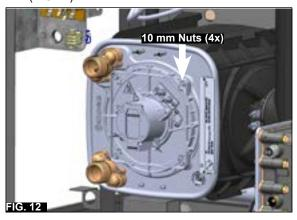
Remove the 'burner and manifold' together. NOTE: BE CAREFUL NOT TO BEND OR DAMAGE THE IGNI-TION PROBES. (Fig.13-14)
