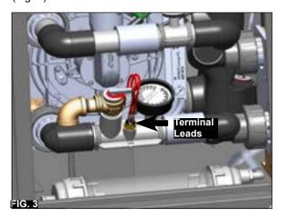
Disconnect the electrical leads from the water pressure switch located on the inlet plumbing assembly (Fig.2).
