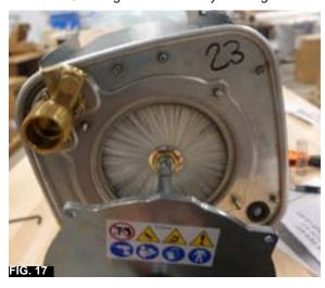
15. Mount the Cleaning Brush flange to the heat exchanger using the 10 mm nuts (x4) that were removed in step 9. The drain plug should be in the 6'o clock position. (Fig. 18-19).
