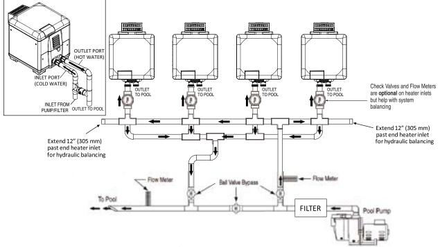
Figure 6. Four MasterTemp® 125 Heaters Plumbing Hydraulic Diagram
