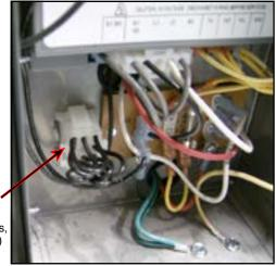
AC Plug 240 Volt (Red wires Top plug)
