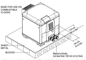
Hollow masonry blocks, not less than 100 mm (4 in) thick, (laid with ends unsealed and joints matched for air circulation). Cover blocks with 0.75 mm (0.03 in) minimum) galvanized sheet metal.
