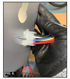
Bring the Flat 5-pin plug, 2 -pin plug into the control box. Install the bushing. If heater has new Control Board bring flame current cable as well. (Fig. 7.)
