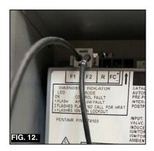
Connect 5-pin connector to lower left side of the ICM. (Fig. 13).
