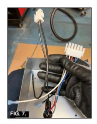
Route the Red and Green wires into the Control Box through the bottom hole. Plug the Fireman's jumper into the terminal board. Install bushing. Be sure the bushings are install when routing the wires into the Junction box. (Fig. 8). Note: The plugs are shown in the control box and the Fireman's jumper installed.
