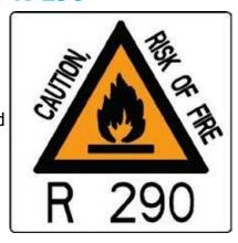
In addition, a *Danger Propane* safety placard should be applied in a visible spot near the service area to alert others that work is in progress and no smoking or open flames are permitted. Instruct everyone in the immediate area as to the nature of the work and safety precautions, and always have an approved fire extinguisher readily available in the vicinity.
