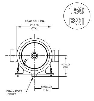
CAUTION: INCORRECT MANIFOLDING WILL CAUSE SEVERE LOCAL STRESS AROUND PORT AND MAY RESULT IN LEAKS AND PREMATURE FAILURE; TAKE EVERY PRECAUTION LISTED ON REVERSE, SEE INSTALLATION
