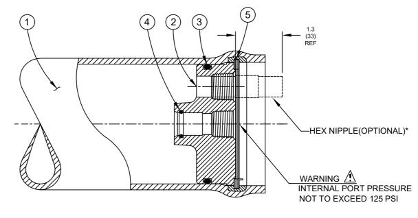
CAUTION: INCORRECT MANIFOLDING WILL CAUSE SEVERE LOCAL STRESS AROUND PORT AND MAY RESULT IN LEAKS AND PREMATURE FAILURE; TAKE EVERY PRECAUTION LISTED ON PAGE 02, SEE INSTALLATION INSTRUCTIONS FOR FURTHER DETAILS
