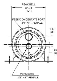
CAUTION: INCORRECT MANIFOLDING WILL CAUSE SEVERE LOCAL STRESS AROUND PORT AND MAY RESULT IN LEAKS AND PREMATURE FAILURE; TAKE EVERY PRECAUTION LISTED ON PAGE 02, SEE INSTALLATION INSTRUCTIONS FOR FURTHER DETAILS
