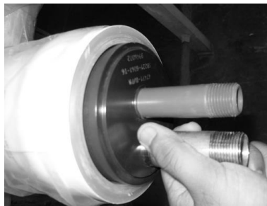
Removal of Head Assembly
