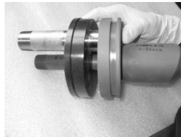
Installing the Bearing Plate and Sealing Plate
