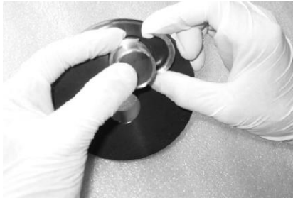
Installing F/C Port & Port Retainer Set
