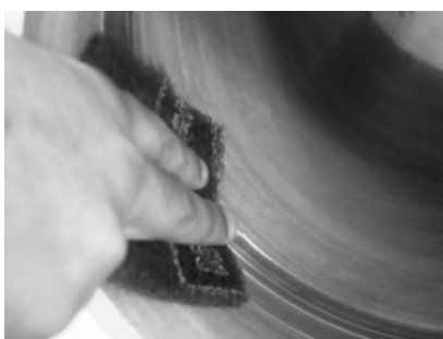
Cleaning inside the vessel
