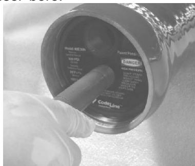
Installation of the End Plug Assembly into the vessel
