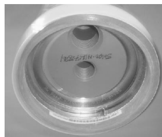
Retaining ring seated in the groove
