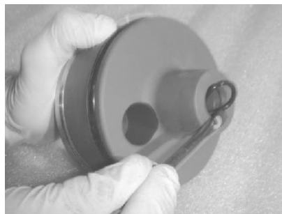
Removal of the PWT Seal
