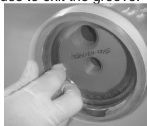
Removal of Retaining Ring
