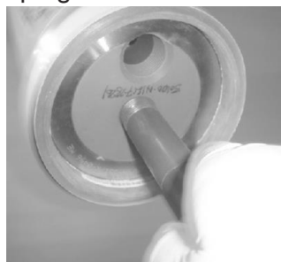
Installation of the End Plug Assembly into the vessel
