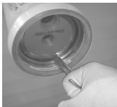
Retaining Ring Removal Tool
