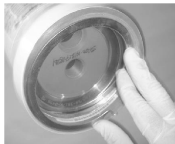
Inserting Retaining Ring into the groove
