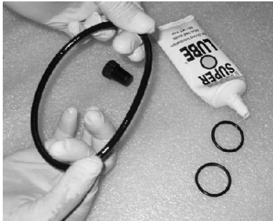
Lubricating Plug seals and O-rings
