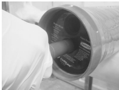
Installation of the End Plug Assembly into the vessel
