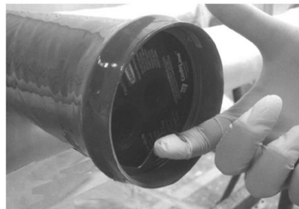
lifting end of retaining ring out of groove
