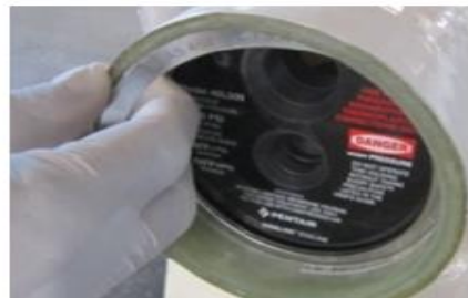
Inserting Retaining Ring into the groove
