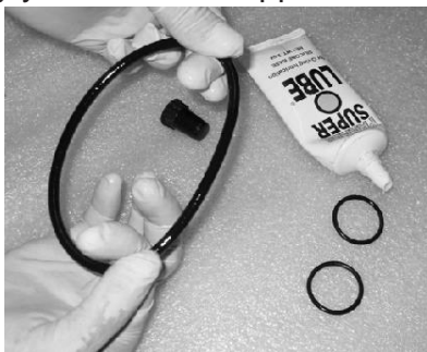
Lubricating Plug seals and O-rings
