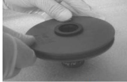
Installing Sealing Plate
