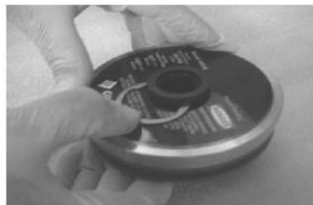
Installing Port Retainer
