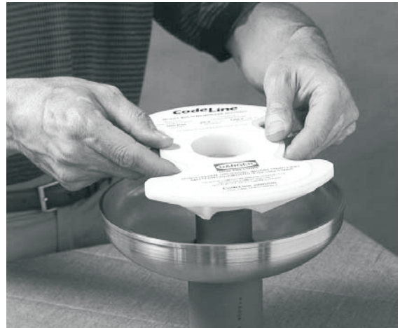
Installing the securing plate
