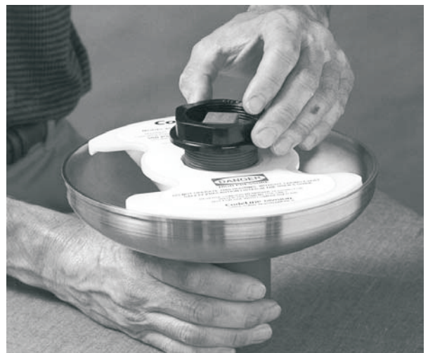
Installing port retaining ring
