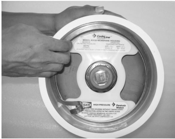
Installing Retaining Ring
