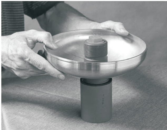
Installing Permeate port
