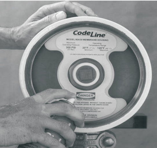
Applying penetrating fluid
