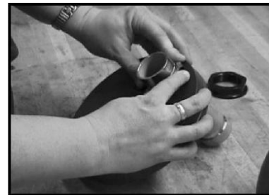
Removing port retainer set
