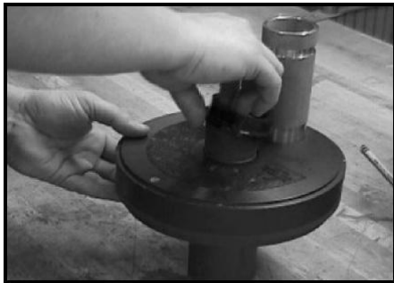
Removing the Permeate Port (left hand threaded)
