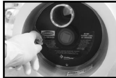
Lifting end of retaining ring out of groove
