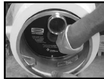
Removing the retaining ring from the groove
