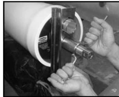
Removing Head Assembly using Head Removal Tool
