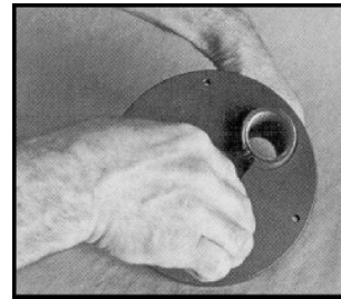
Port being fitted using snap ring pliers
