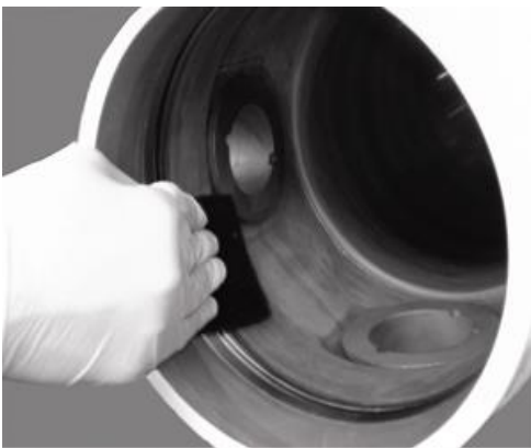
Cleaning inside the vessel
