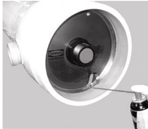
Applying penetrating fluid
