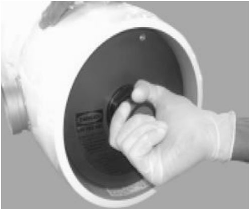
Installing Head Assembly
