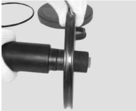
Installing Sealing Plate
