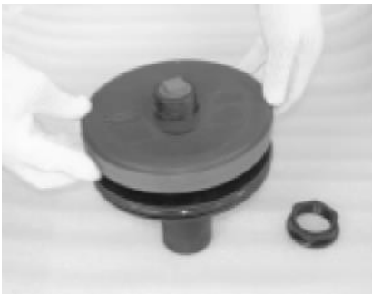
Removing the Bearing Plate
