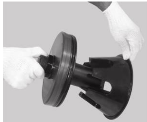
Installing Thrust Cone
