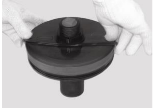
Installing Head Seal
