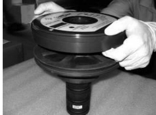
Installing Bearing Plate
