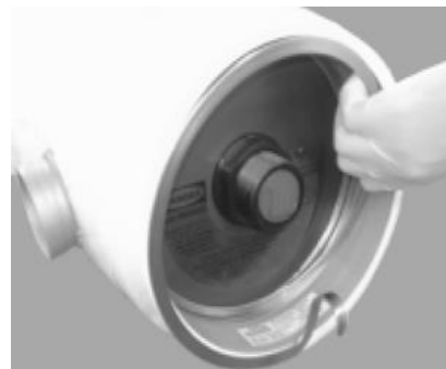
Removing the retaining ring from the groove
