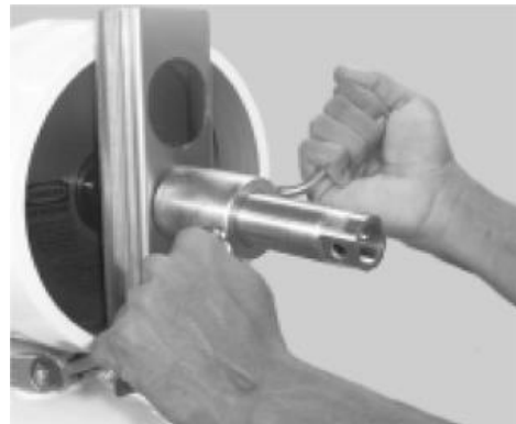
Removing Head Assembly using Head Removal Tool
