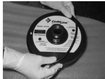
Installing Head Seal
