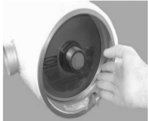
Installing Head Retaining ring
