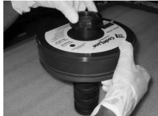
Installing Port Nut
