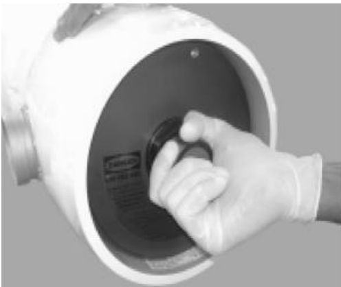
Installing Head Assembly
