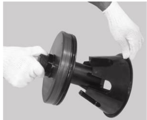
Installing Thrust Cone
