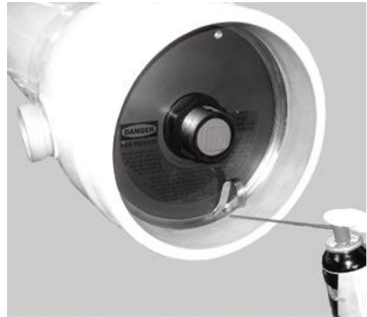
Applying penetrating fluid
