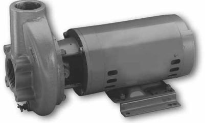
The CC Series Pumps are compact and lightweight, but rugged. Choose from 3 or 5 HP high head and medium head models. For lower pressures and maximum capacity, medium head models offer heads to 75 feet and capacities to 220 GPM. Where higher pressures are desired, the high head model offers heads to 102 feet and capacities to 260 GPM. Optional Flange and Trap Packages Available
